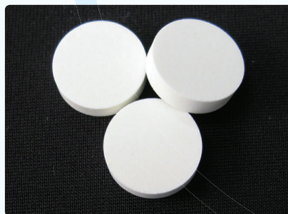
Linseed oil tablet, Ø11.3mm, 125N at 500 kg/cm 2
